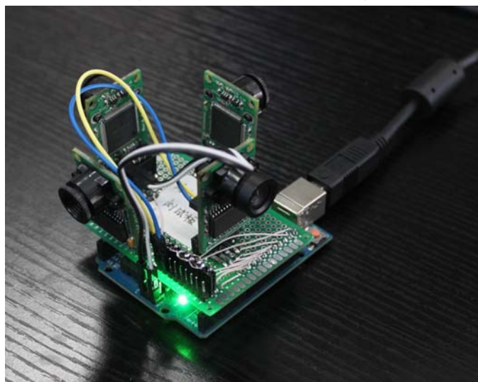
Figure 4 Multi-Cameras Wiring on Arduino UNO
